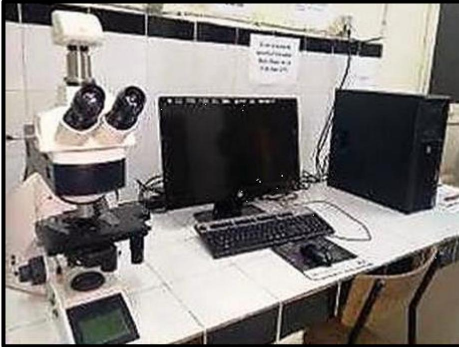
**Figure 9:** Microscope photonique LEICA DM4000 B LED.
